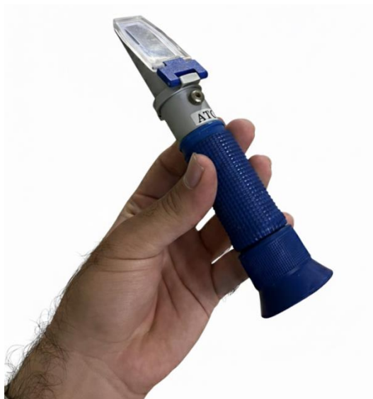
Figure 1: Handheld optical refractometer (Model HRB90-T, A.Krüss Optronic, Germany) featuring a 0–90% Brix scale and an integrated thermometer (6–36°C) used for analyzing serum samples. Photograph by Saeed Kashi
